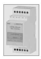
Its output becomes active (closing the open contact and opening the closed one) when the well water level reaches the maximum level, keeping this position until de level descends below the minimum. Due to this reason, its main application is the pumps protection through its normally open contact (it closes only if there is water), and the indication of lack of water or opening of electro-valves of filled control, through its usually closed contact.
